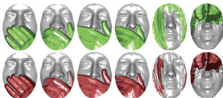
FIGURE 2.12 – Highly occluded sample images that are correctly classified by the proposed masked Fisherfaces approach from the Bosphorus dataset. Top and bottom rows show the corresponding manually labeled (in green) and automatically detected (in red) occlusion masks. Alyuz et al. (2013)
