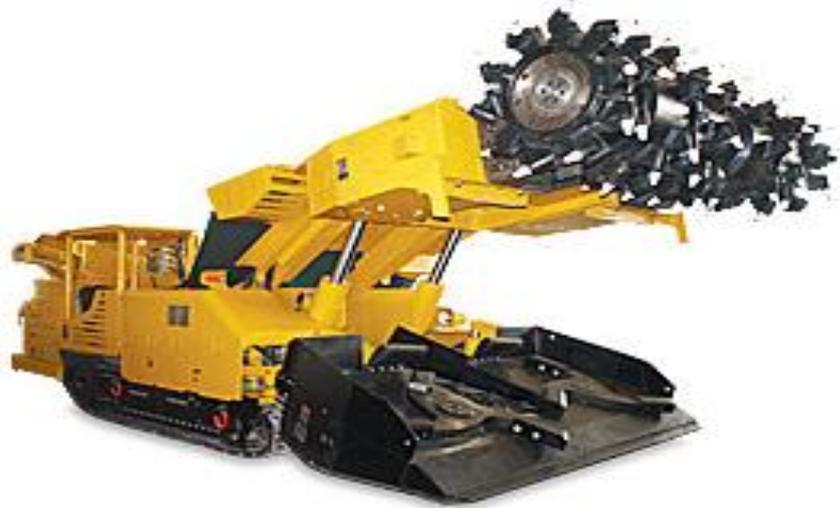
**Figure 2.5. Machine Paurat twin-boom heading - Model PTF70**
