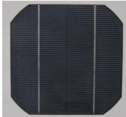
FIGURE 1.9 – Plaque de silicium monocristallin
