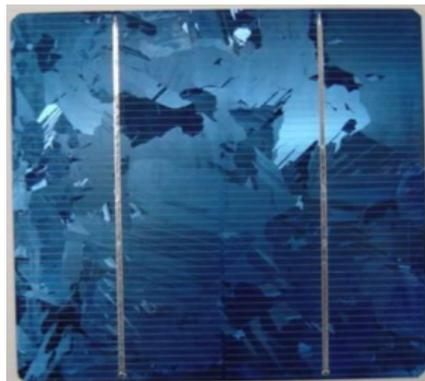
FIGURE 1.10 – Plaque de silicium poly cristallin
