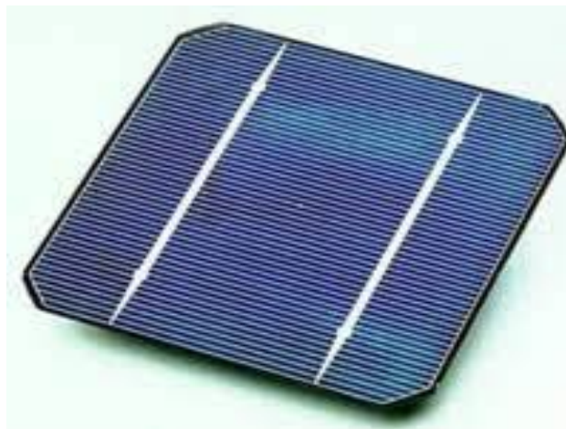
Figure II.2: Plaque de silicium monocristallin.
