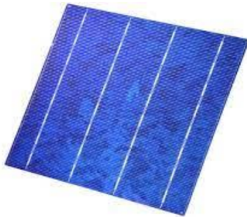
Figure II.3: Plaque de silicium poly cristallin.
