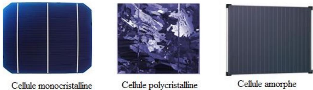
Figure II.2: Types de cellules solaires.
