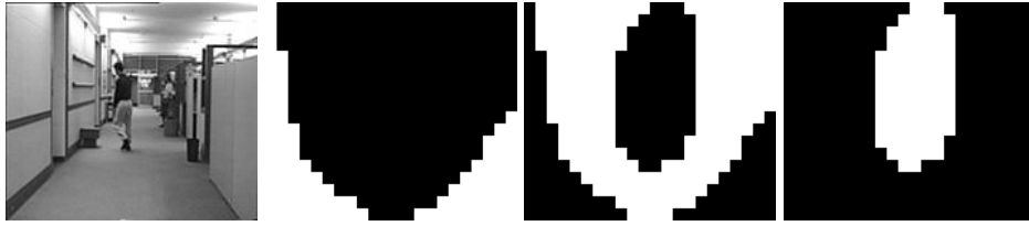
Figure 4.2: Example shows the results of segmentation for the 3 regions, 1-Frame 85 form Hall sequence. 2-Mask of the 3rd ROI. 3-Mask of the 2nd ROI. 4-Mask of the 1st ROI (Th1=0.0224, Th2=0.0301)
