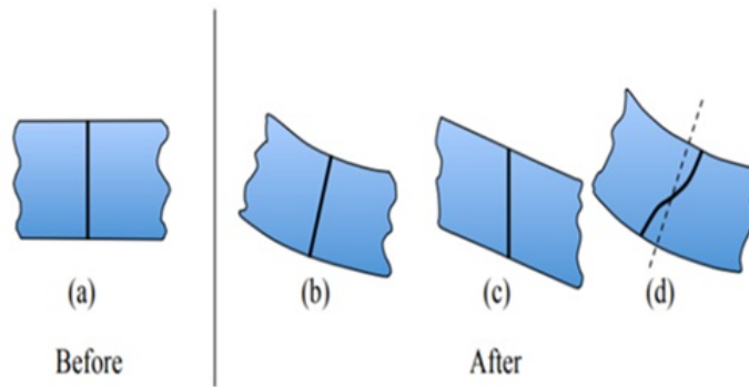
Figure 2.5: Flat (b) and (c) and warped (d) cross-sections after deformations.
