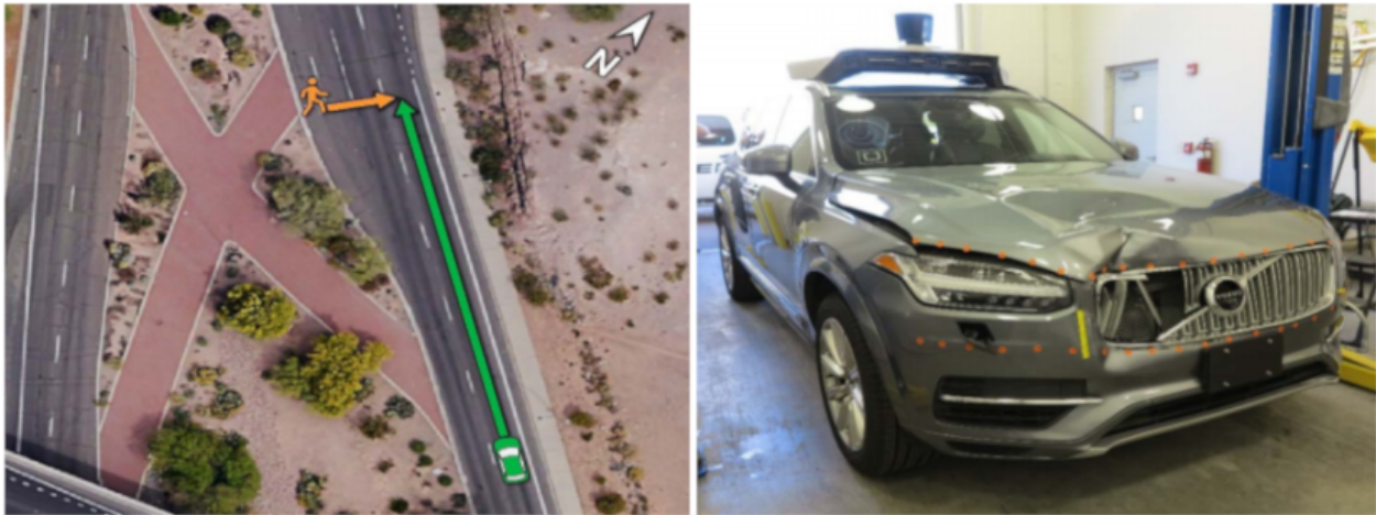
Figure 1.2: (Left) Location of the Uber crash, showing the paths of the pedestrian in orange and of the Uber test vehicle in green. (Right) Post-crash view of the Uber test vehicle, showing damage to the right front side.
