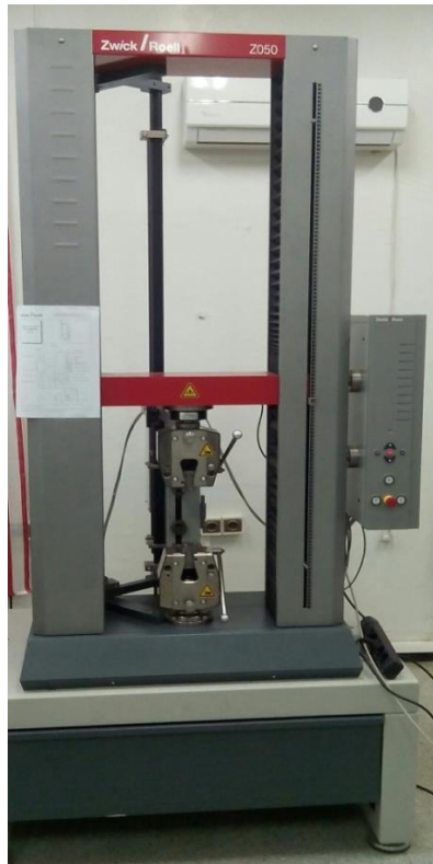
Figure II.13 : La machine de traction de type Zwick.
