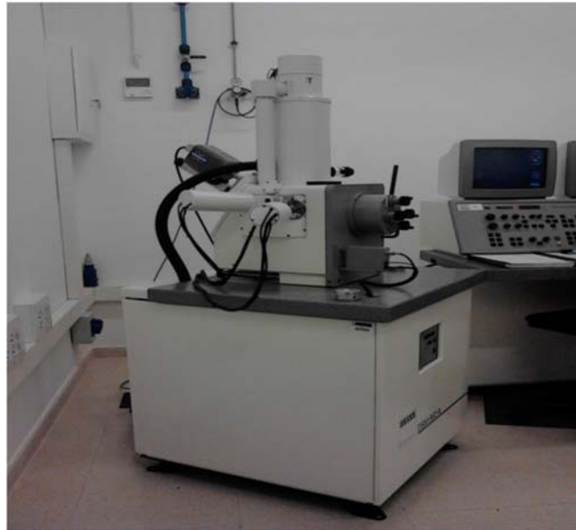
Figure II. 3 : MEB type DSM 960A Zeiss.
