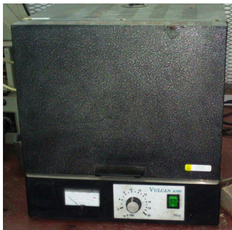
Figure IV.4: Four est VULCAN A-550 [labo department métallurgie annaba ]
