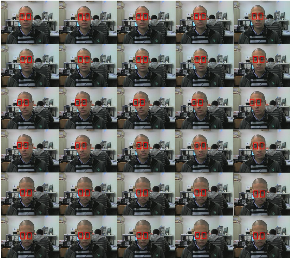
Figure 3.17: Three segment of video sequence demonstrating the success of our detector in real world conditions. The video is recorded inside the research lab with different lighting conditions, head rotation, cluttered background, facial expressions and accessories (e.g., glasses) [147].. (Zooming is recommended for digital visualization).
