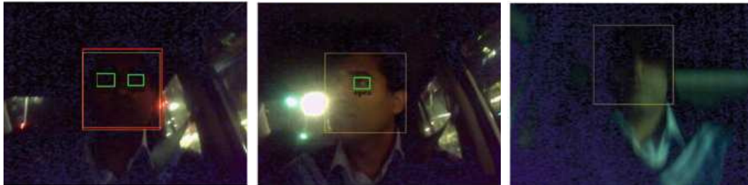
Figure 1.8: Face and eye opening and closing monitoring at night under difficult environmental and imaging conditions: eye detection failure due to motion blur, one eye not located due to face rotation [42].
