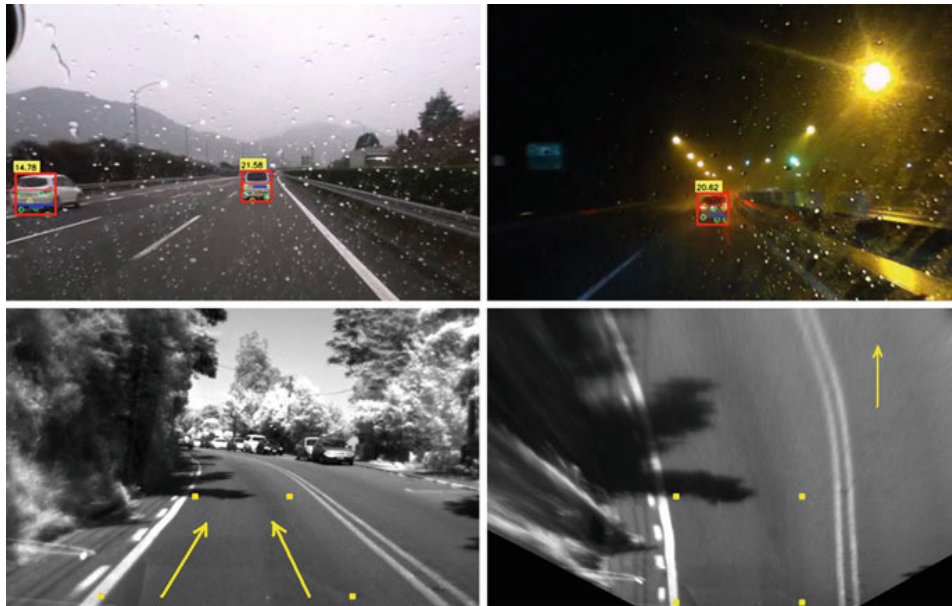
Figure 1.4: In the top row, monocular vehicle detection under challenging environmental and lighting conditions: detected vehicles are also labeled by monocular distance measure. In the bottom row, a transform from perspective view into a bird's eye view employed for monocular distance measures. [42]
