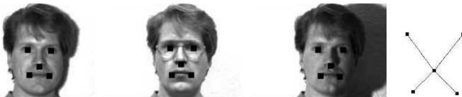
Figure 3.5: Three illustrations of the training set indicating the position of the marked features and the structure of the pictorial model learned [111].
