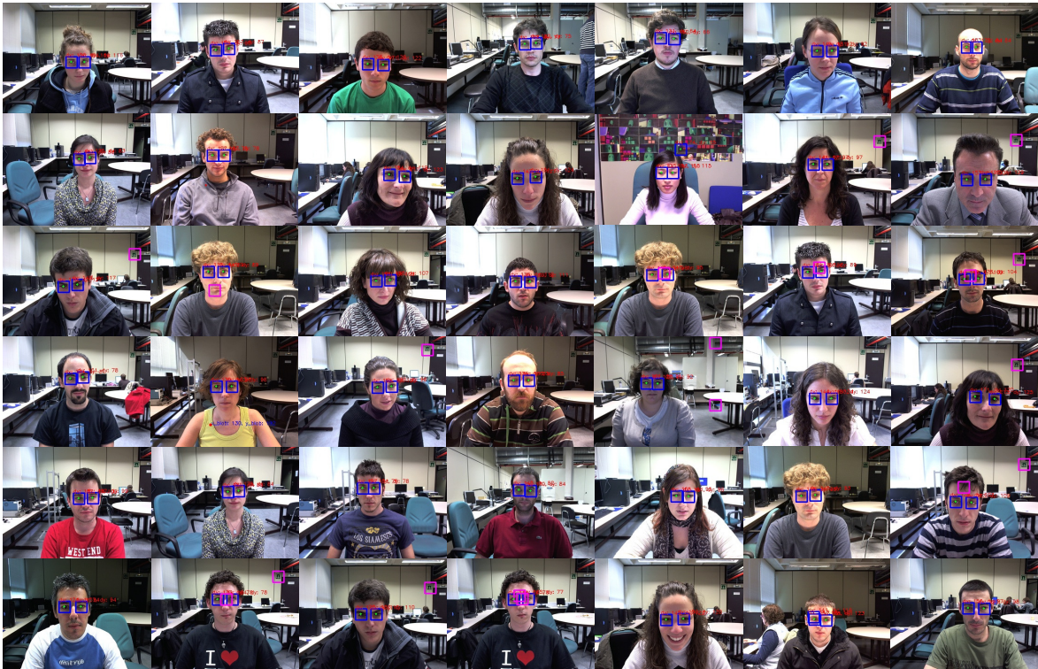
Figure 4.3: Results of the analysis of the eye location by the EyeLHM [186] system that validates threshold value for an accurate detection of the eye under difficult conditions of GI4E dataset: the blue rectangles represent the precise eye location, the magenta rectangles are the false positives rejected from similarity measure, the green points represent the center of the eye detection.
