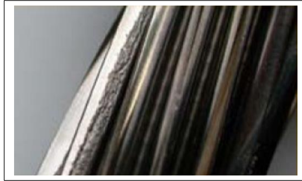
Figure 1.24 Ecaillage des dents.
