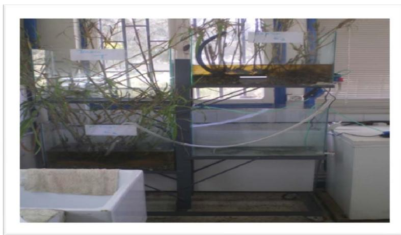
**Fig. 1:** System of purification (two stages of purifications). (*Laboratory of Cellular Toxicology*)
