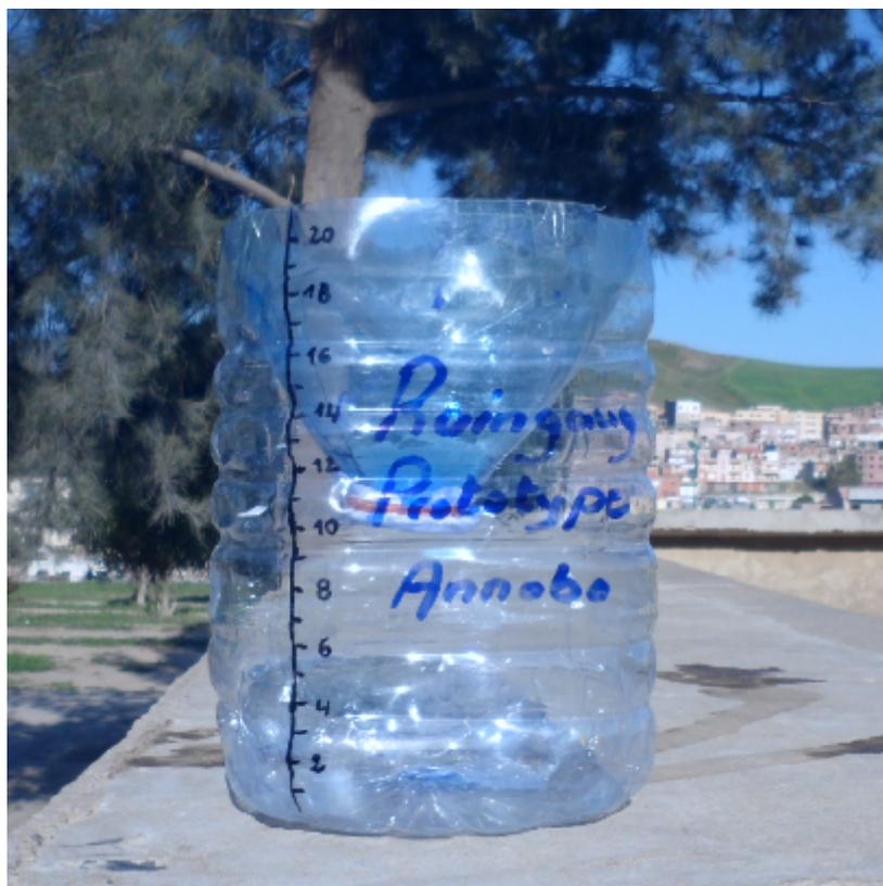
**Figure 16:** Rain gauge sampler used in the Annaba region during the period 2011-2013.
