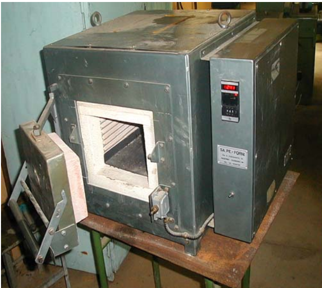
b)- Four SA-PE Type RN-14, P=4.5 kW, 7 Ampère, T° max. 1100°c
