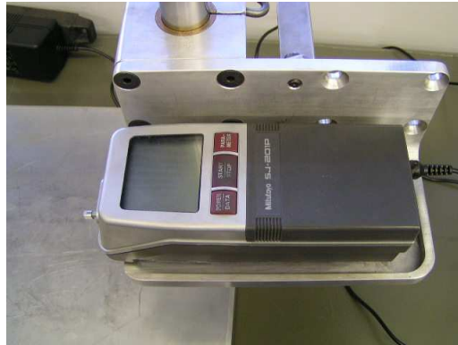
Figure II.9 - Rugosimètre Mitutoyo SJ 201.M.
