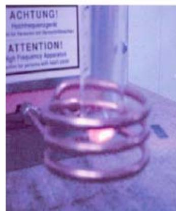
Figure II-6. Alliage Al-( $\alpha$ -Al<sub>2</sub>O<sub>3</sub>) en fusion.
