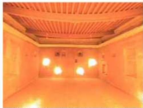
After 90 minutes test - distortion of the structure
