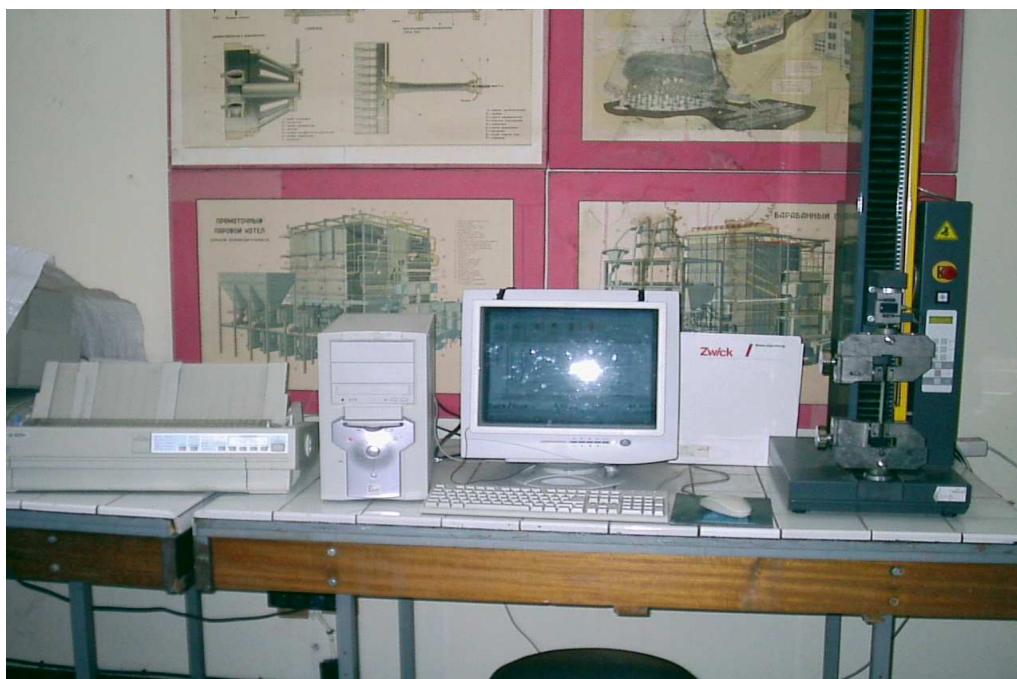
Figure. III.04 Machine de traction Zwicky 1120 (LR3MI)
