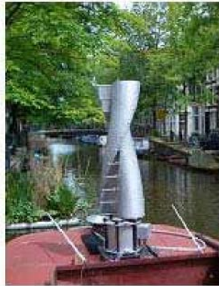
Figure 1.5 : Eolienne de type Savonius (Wind Side) [17]
