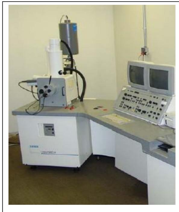
Figure II-11. Photo du MEB type DSM Zeiss 960 A [32].
