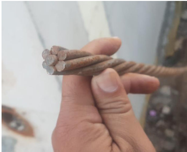
Figure 4 : strand with 7 wires.
