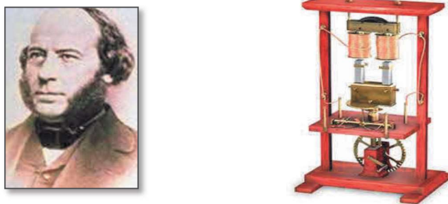
Fig 6.4 Commutator-type DC generator (dynamo), developed by Hippolyte Pixii
