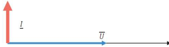
Fig. 2.23 Capacitor ; voltage and current vectors
