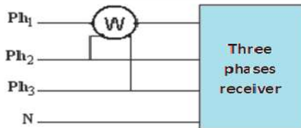
Fig.3.23 Measure reactive power using a single wattmeter
