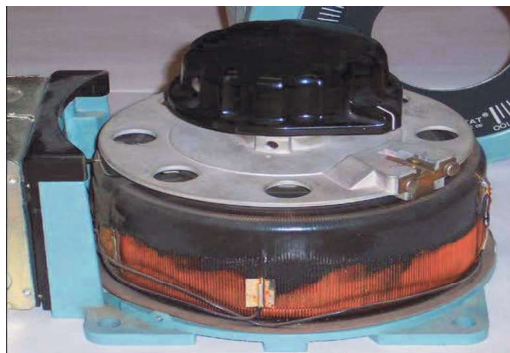
Fig.5.8 Variable ratio auto transformer
