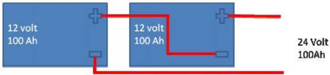
Figure 3.4.2.1 Series configuration of batteries
