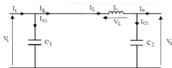
**Fig. III.5:** Buck Converter – Switch Closed
