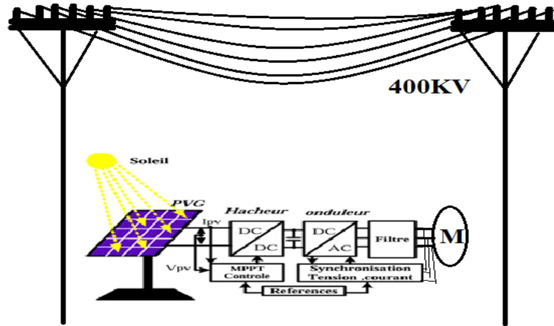
**Fig. III.1:** Block diagram of an off-grid PV system
