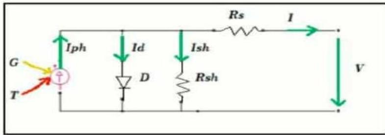
**Fig. III.3:** Equivalent circuit diagram of a photovoltaic cell
