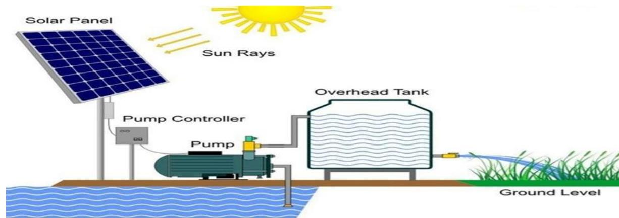
**Fig. II.14:** Diagram of a Photovoltaic Pumping System
