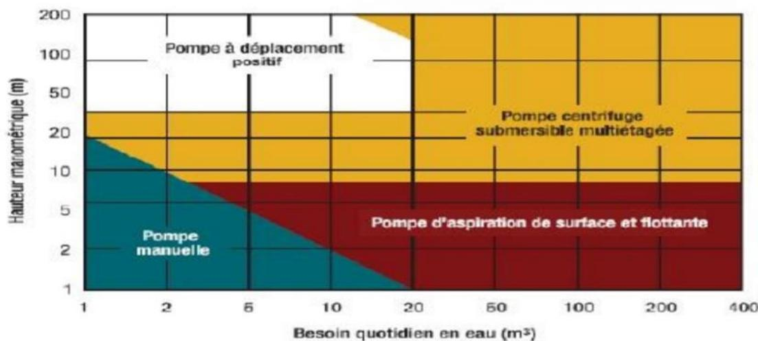
**Fig. II.15:** Pump Type Selection
