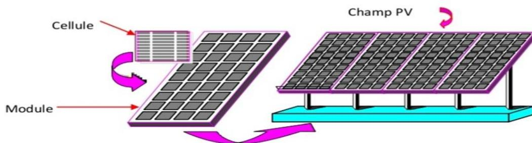
**Fig II .9:** Components of a photovoltaic generator
