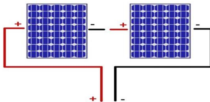
**Fig. II.10:** Series Connection of Solar Panels
