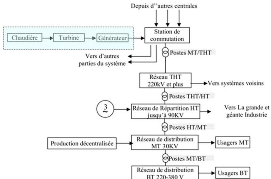
**Fig. I.1:** Configuration of the electro-energy system
