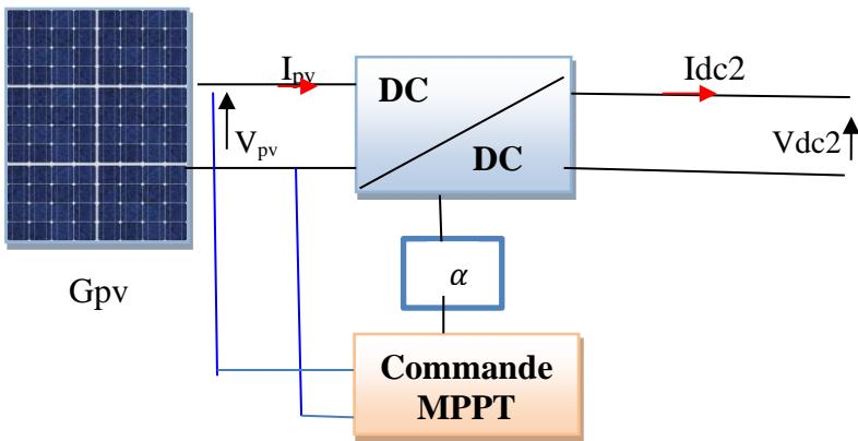
**Fig. III.14:** Basic Chain of a Photovoltaic System with a Converter
