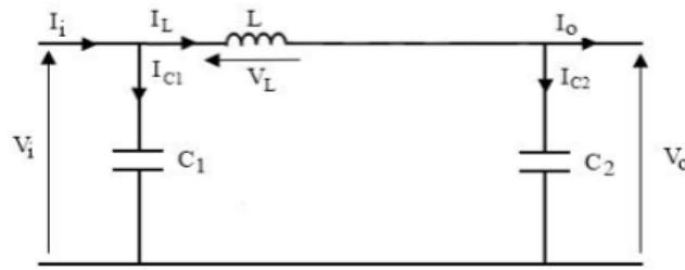
**Fig. III.9:** Boost Converter – Switch Open
