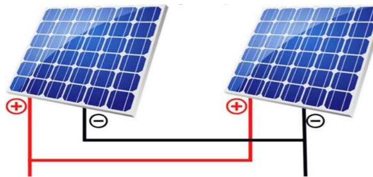
**Fig. II.11:** GPV Mixed Connection
