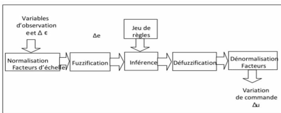
**Fig. III.13:** Structure of a Fuzzy Controller
