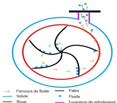
**Fig. II.17:** Difference Between Centrifugal Pump and Volumetric Pump Rotary Volumetric Pumps
