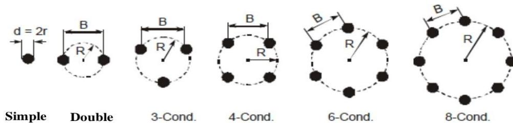
**Fig. I.6** : Configuration of bundled conductors for HV and THT lines
