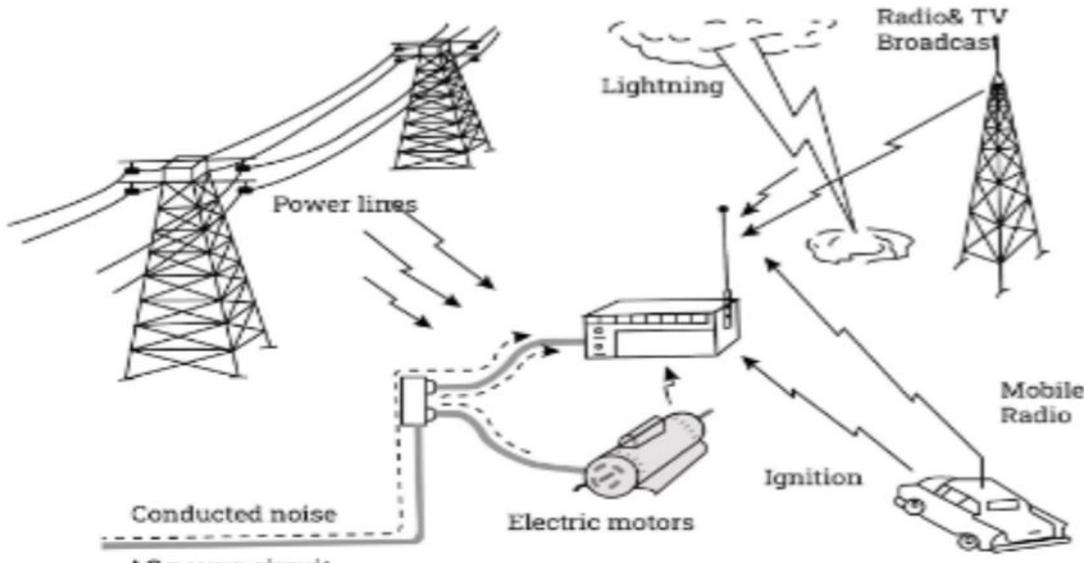
**Fig. I.8 :** Different sources of electromagnetic fields
