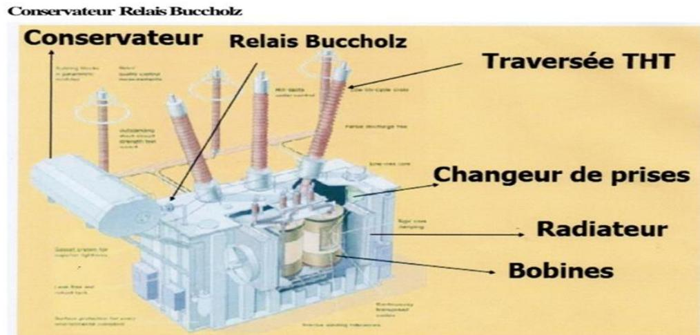
**Fig. I.4 : Cross-section of a transformer**
