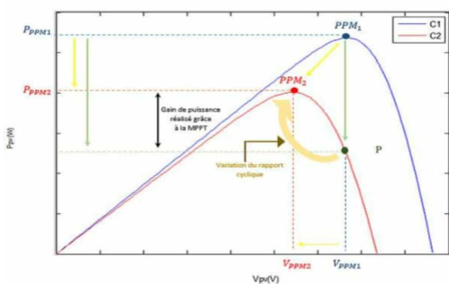
**Fig. III.15:** Tracking and Recovery of the Maximum Power Point (MPP)
