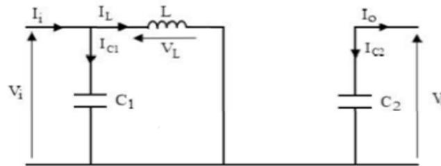
**Fig. III.8:** Boost Converter – Switch Closed
