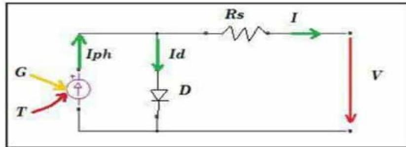
**Fig. III.2:** Equivalent circuit diagram of an ideal cell
