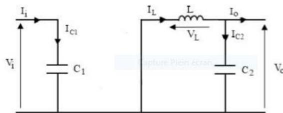
**Fig. III.6:** Buck Converter – Switch Open
