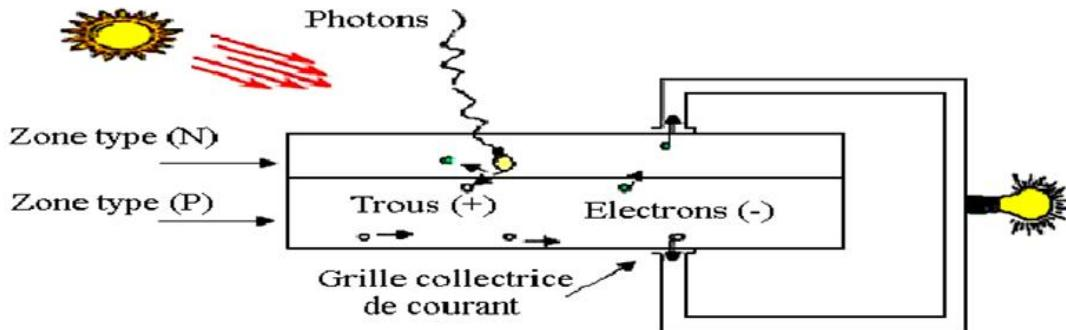
**Fig. II.13:** Explanation of the Conversion Principle in PV Systems
