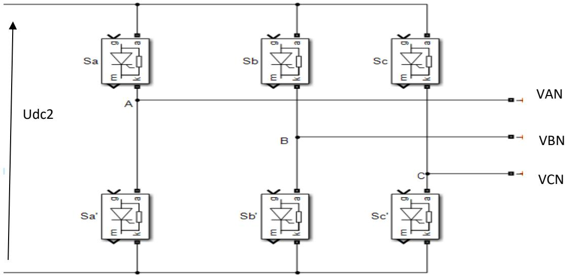
**Fig. III.11:** Structural Diagram of a Two-Level Three-Phase Inverter
