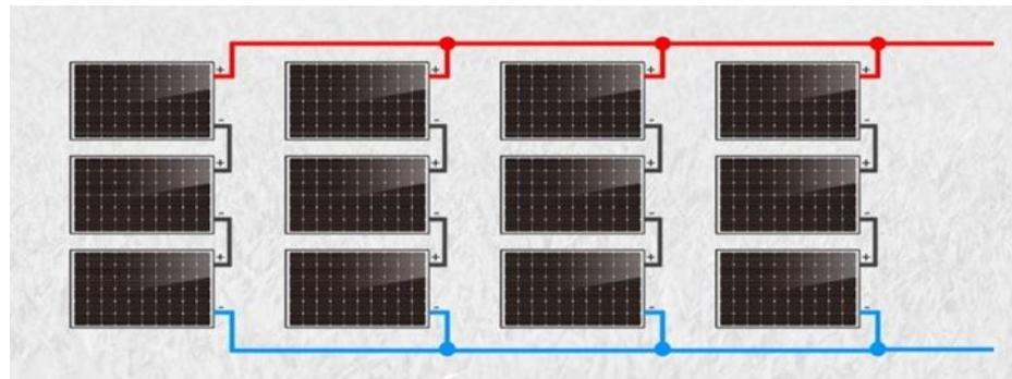
**Fig. II.12:** Hybrid Configuration
