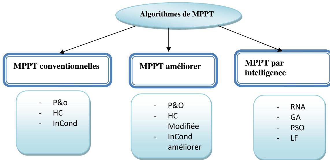
**Fig. III.17:** Classification of MPPT Methods
