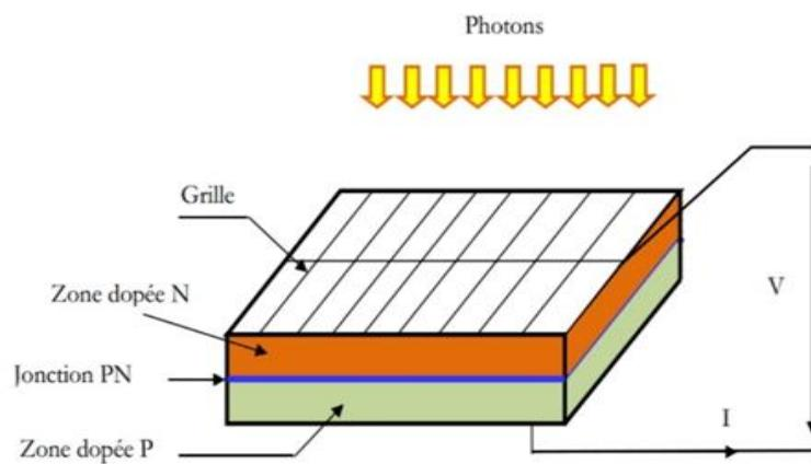
**Fig II.8 :** Structure of photovoltaic cell
