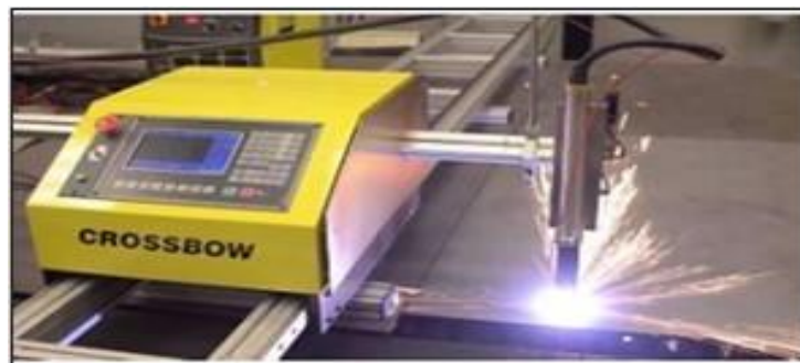
fig.1.8: CNC plasma cutters [5].
