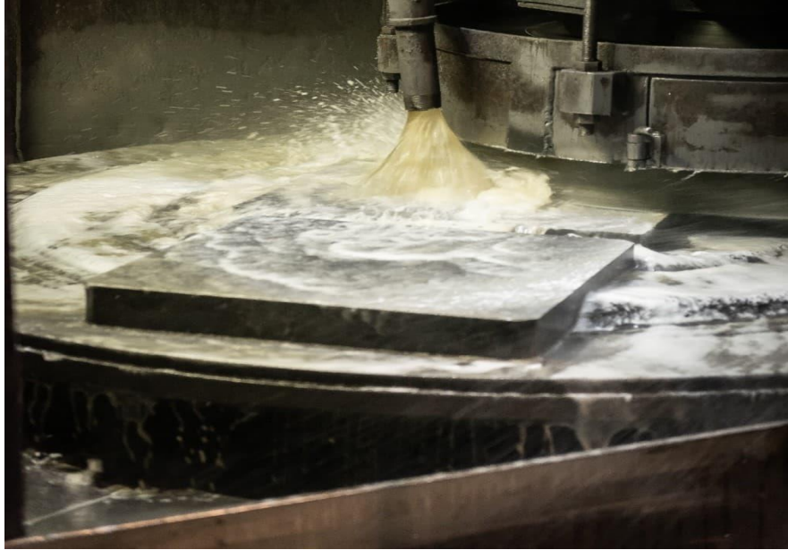
Figure II.19: Rectification plane de type Blanchard. [20]
