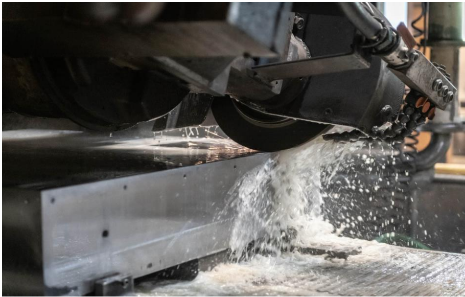
Figure II.20: Rectification plane tangentielle grande dimension. [20]
