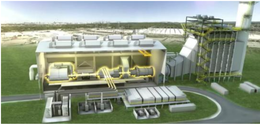
Fig I.3. View of the layout of a combined cycle.
