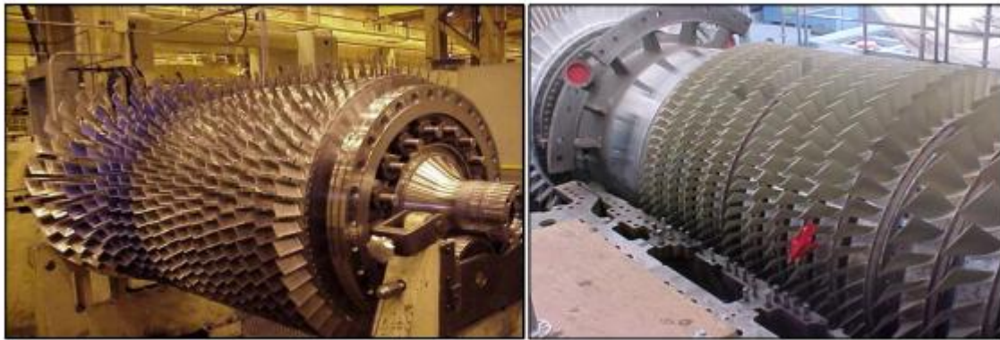
Fig I.10. View of the 18-stage compressor rotor.
