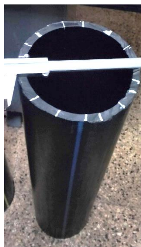
Figure II.1: HDPE-100 Pipe Used for Sample Preparation
