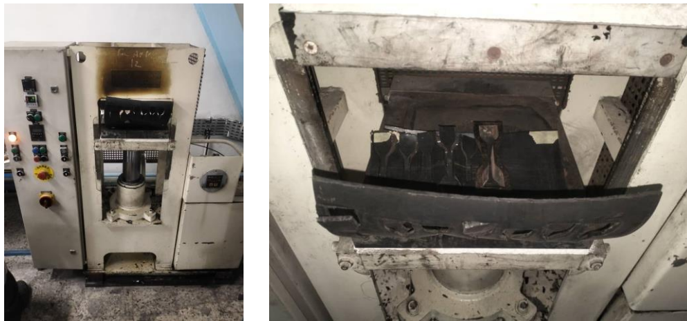
Figure II.16: The hydraulic press (used to cut the specimens)
