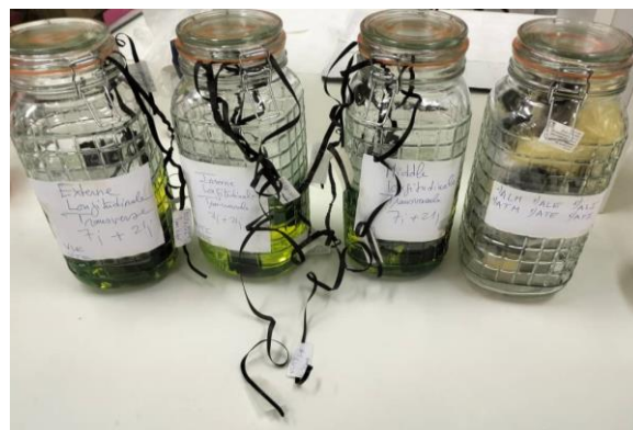
Figure II.21: Glass Containers Used for Specimen Immersion
