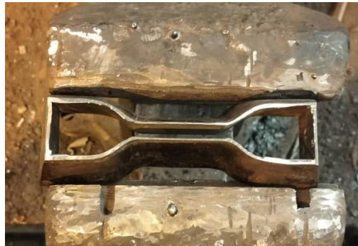
Figure II.15: The die used to cut the specimens
