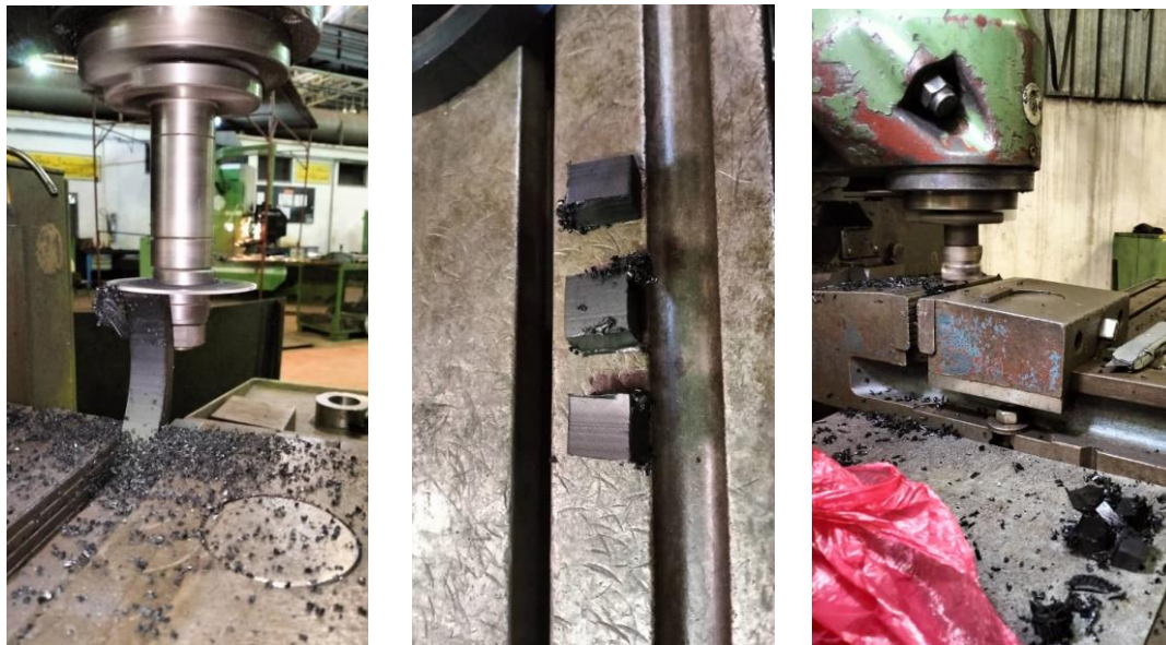
Figure II.24: Fabrication of Parallelepiped Samples Using a Milling Machine
