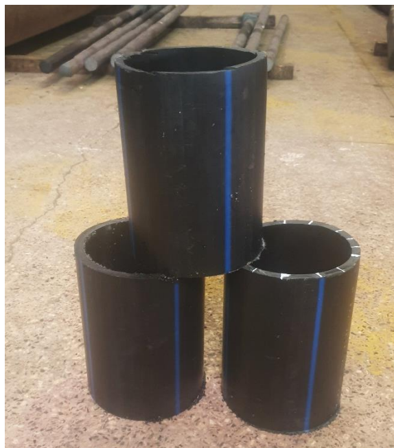
Figure II.3: The three pipes pieces obtained after cutting (similar cylinders)
