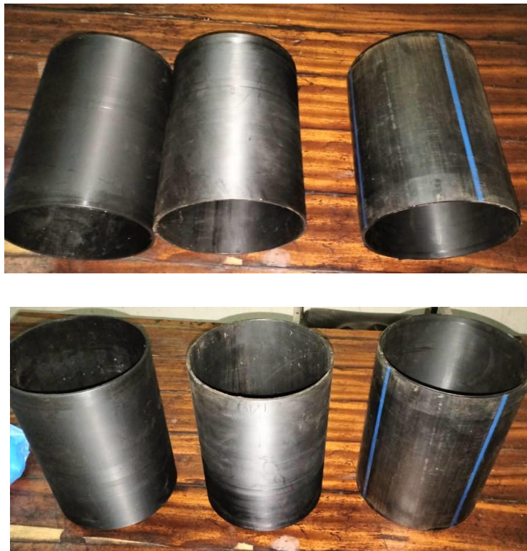
Figure II.5: The three obtained pipes (inner, middle, outer layers)
