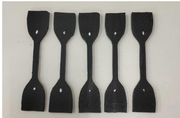
Figure II.22: Specimens Undergoing Preparation for Tensile Testing
