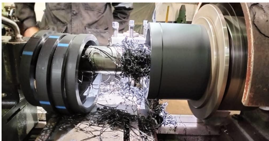
Figure II.23: Ring Cutting Process on the Lathe
