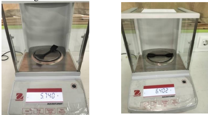
Figure II.19: Weighing L and T Specimens with a High-Precision Balance
