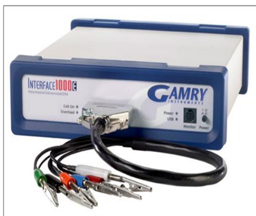
Figure 9. Potentiostat marque Gamry interface 600
