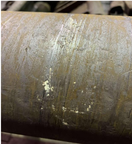
Figures V.6. Fissure transversale
