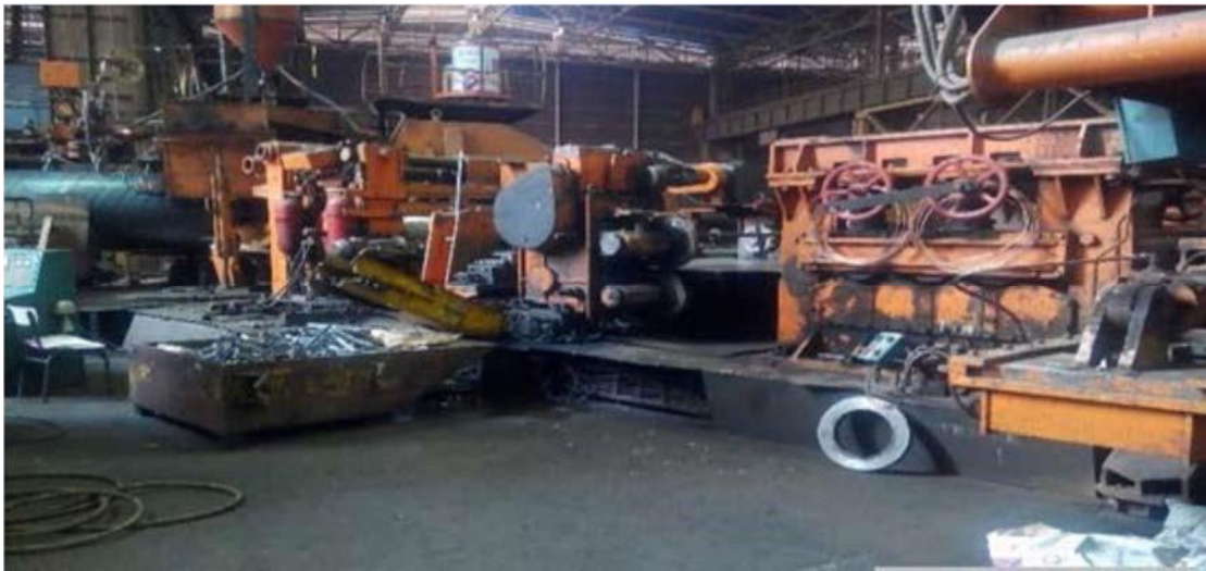
Fig.I.7 : Machine (planing, guiding, strip dressing, shearing)
