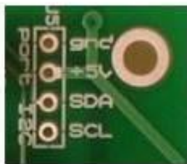
Fig-4.16 I2C Port on POB-Proto
