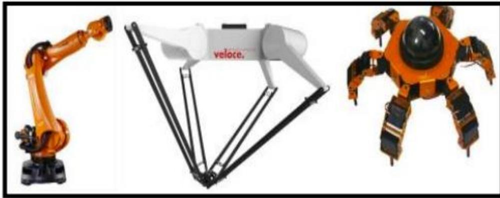
***Figure 1.1*** (a) Robot Kuka, (b) Robot Delta, (c) Robot hexapode
