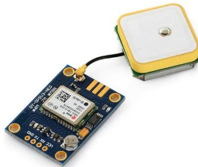
Figure II.4: Module GPS (NEO-6) [6]
