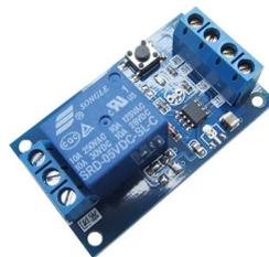
FIGURE 4.11 – Module de relais Bistable 5V
