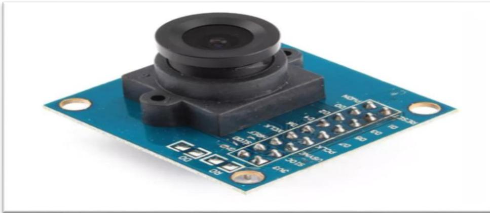
**Figure 25 :** Module Camera OV7670
