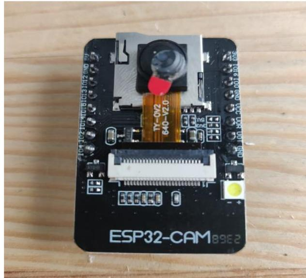
*Figure II.1 CARTE DE DÉVELOPPEMENT ESP32-CAM*
