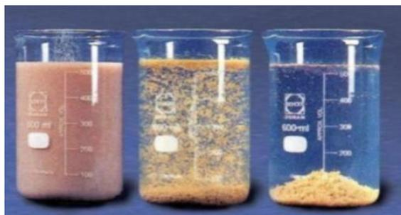
Figure I- 7: coagulation et floculation
