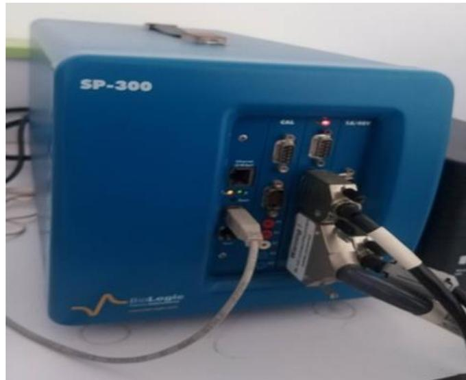
**Figure IV.4. Potentiostat / Galvanostat SP300.**
