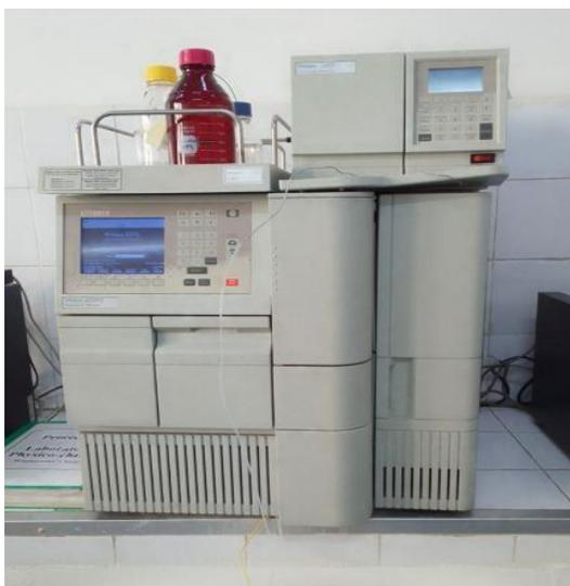
**Figure I.21.** Appareillage de HPLC (Waters Alliance 2695)
