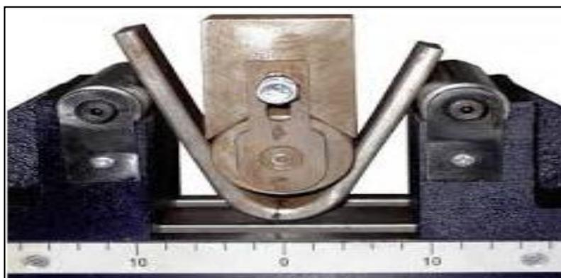
Figure I.13: Essai de pliage.
