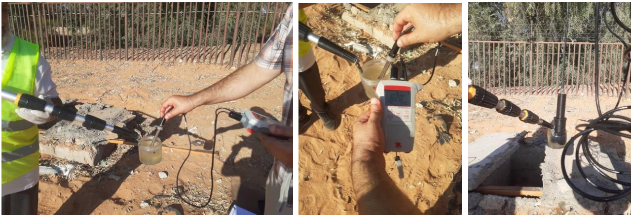
Figure 26 .In situ of parameters (pH- conductivity, temperature and SS)
