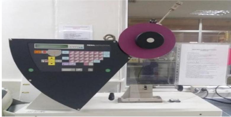
**Figure IV-20:** Appareil IZOD
