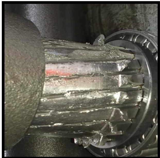
Figure II.15 pignon (e) cassé.
