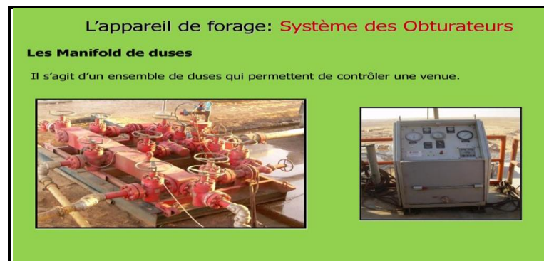
Figure I.30: Manifold duses (Choke Manifold).
