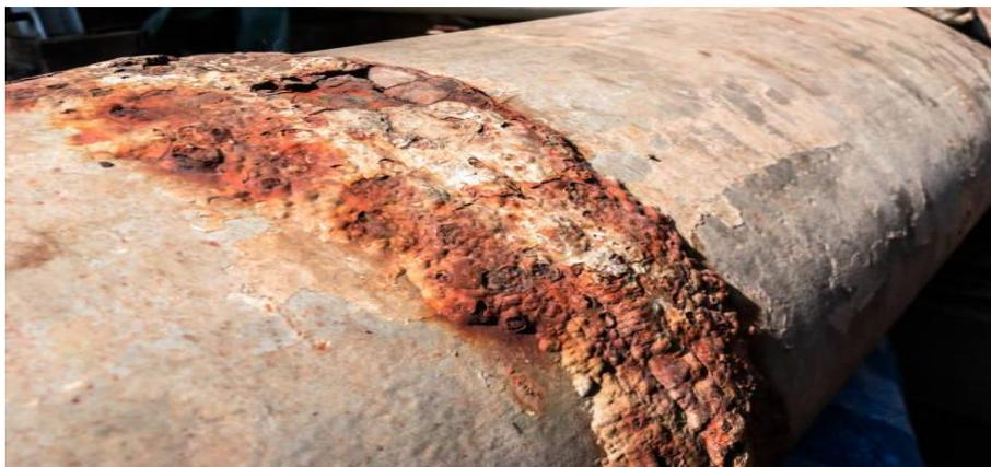
Figure 36 corrosion externe
