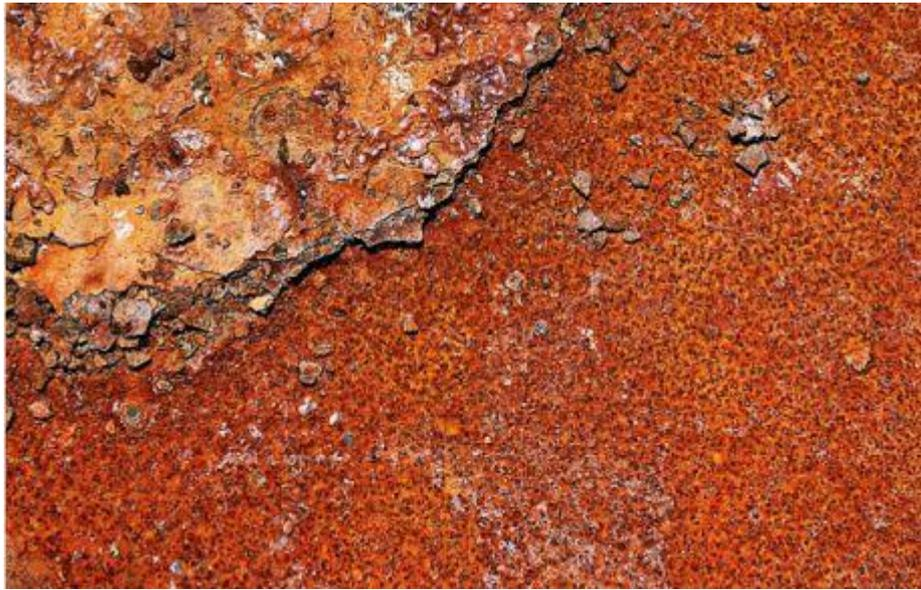
Figure 37 Corrosion uniforme
