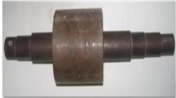
**Figure I. 5-**Rotor massif lisse
