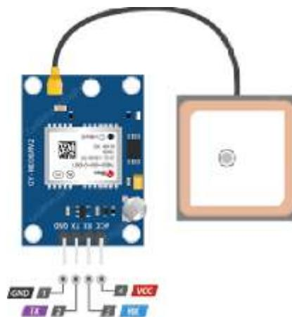
Figure III.12- Module GY-NEO6MV2
