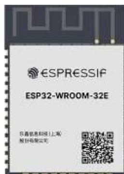
**Figure III.2 ESP32 WIFI /Bluetooth Low Energy Module [20]**
